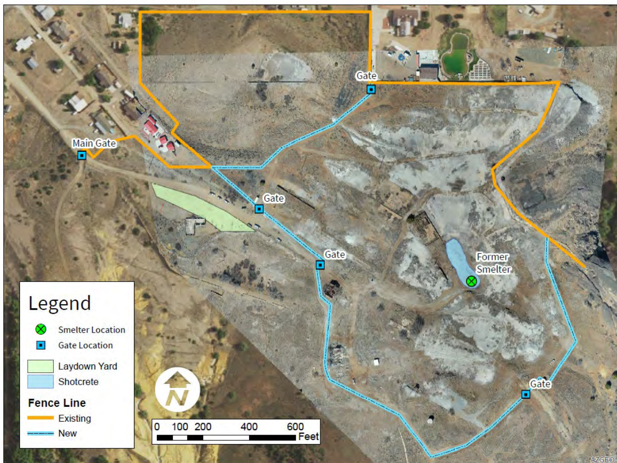
Figure 2. Existing and New Fencing
