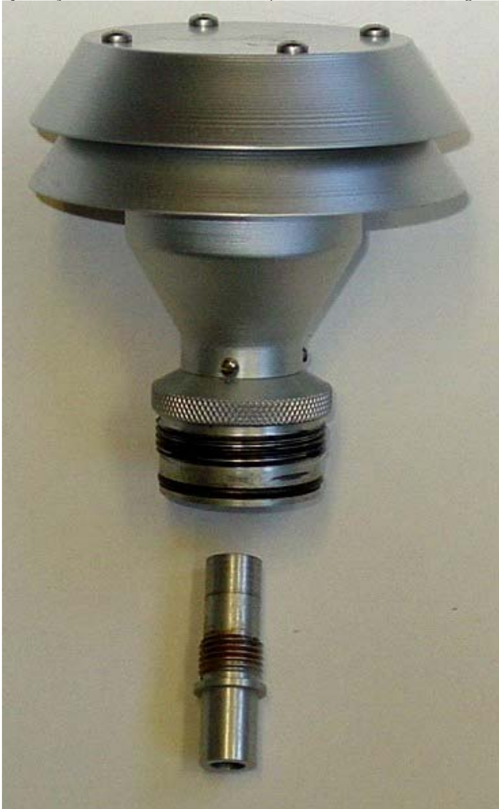
Figure 11: Photo of Jet Removed for Cleaning or Size Change
