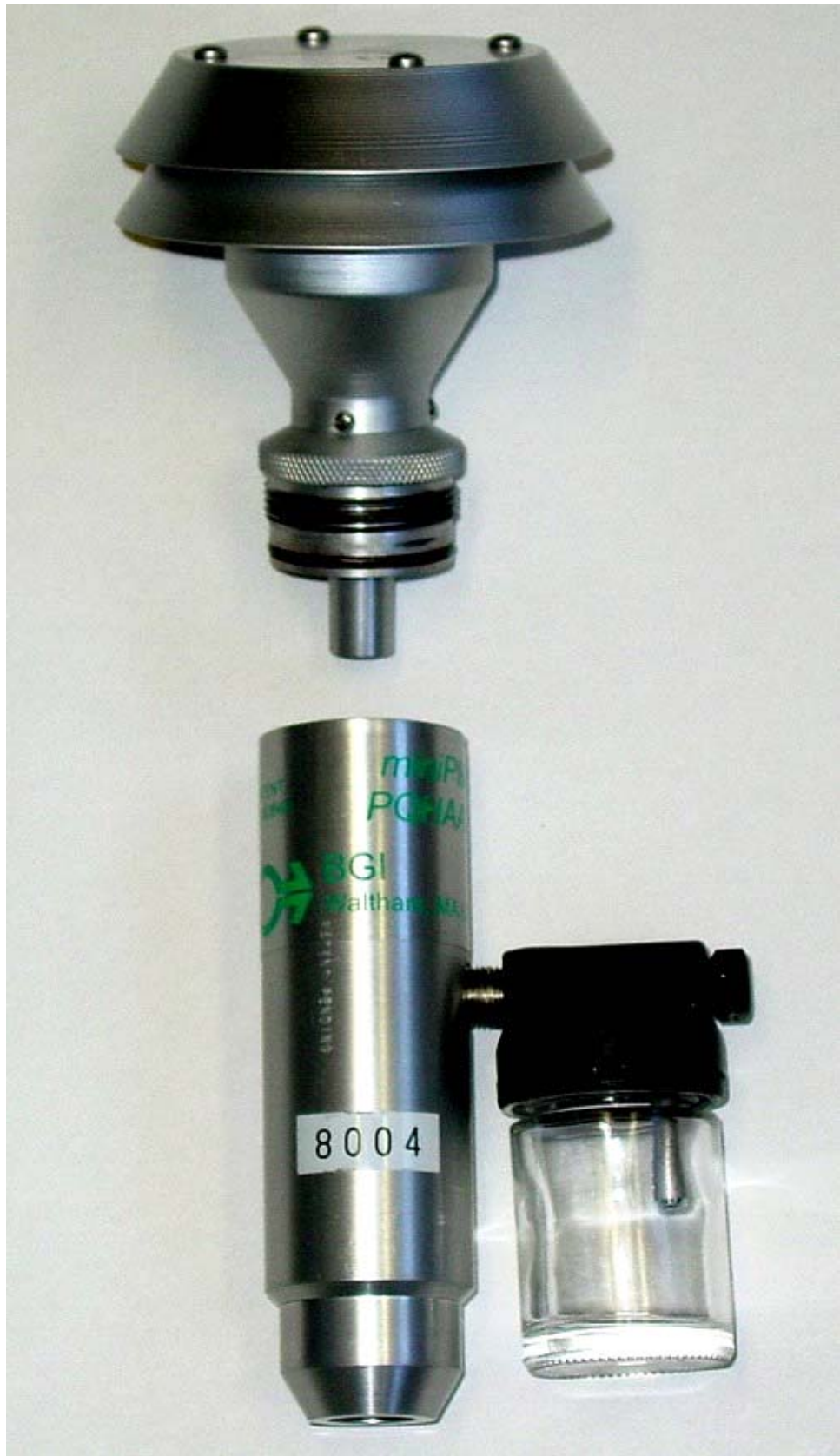
Figure 10: Photo of Initial Disassembly of Inlet
