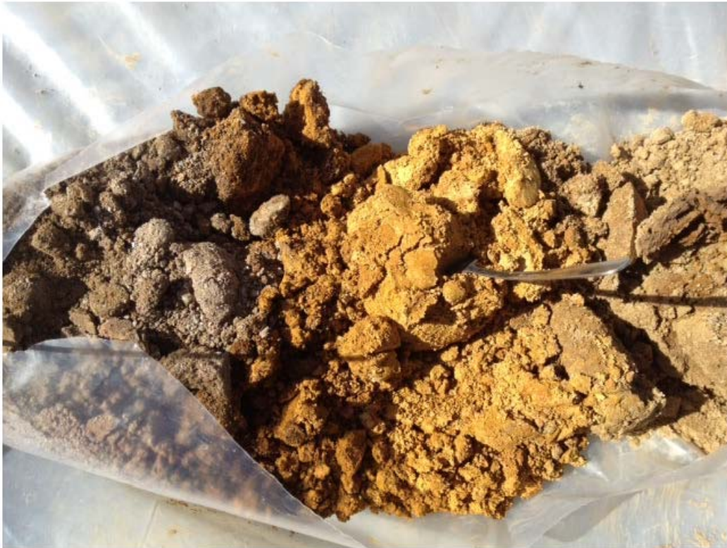
Photo 1: Part of a core into the Tailings Floodplain showing yellow-orange oxidized tailings layer on top of other deposit material
