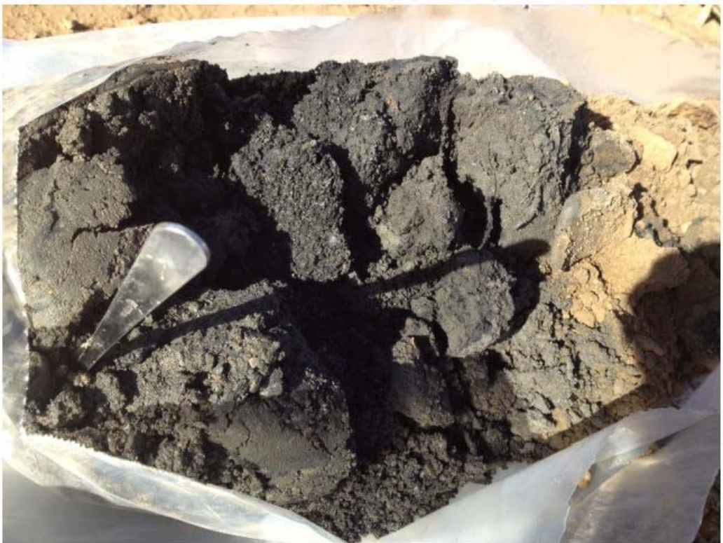
Photo 2: Part of a core into the Tailings Floodplain, showing black reduced (anoxic) tailings
