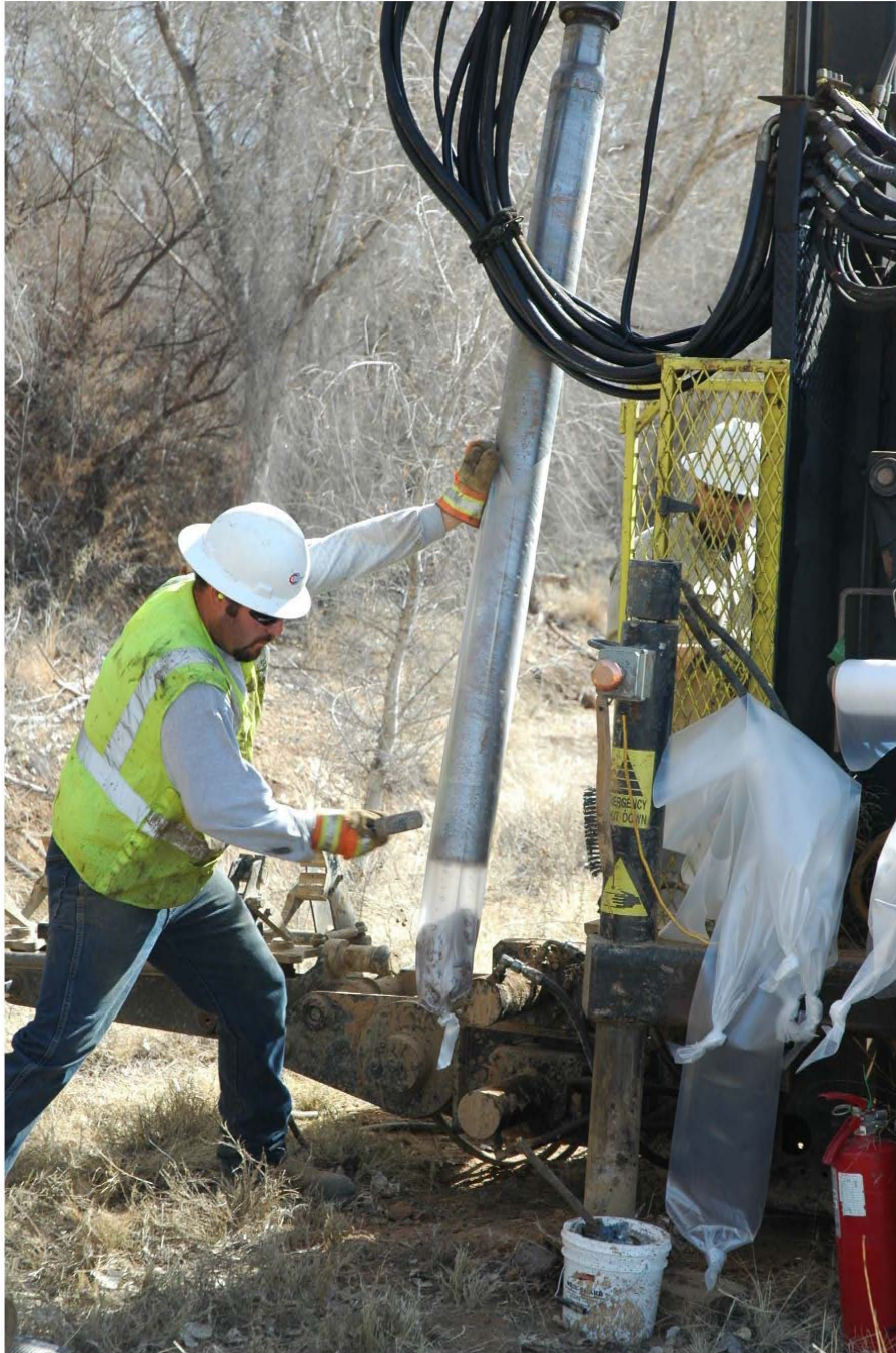
Photo DSC_0615: Photos during investigation: depicting percussion drill rig used to obtain cores from the ground in area of the Humboldt Smelter
