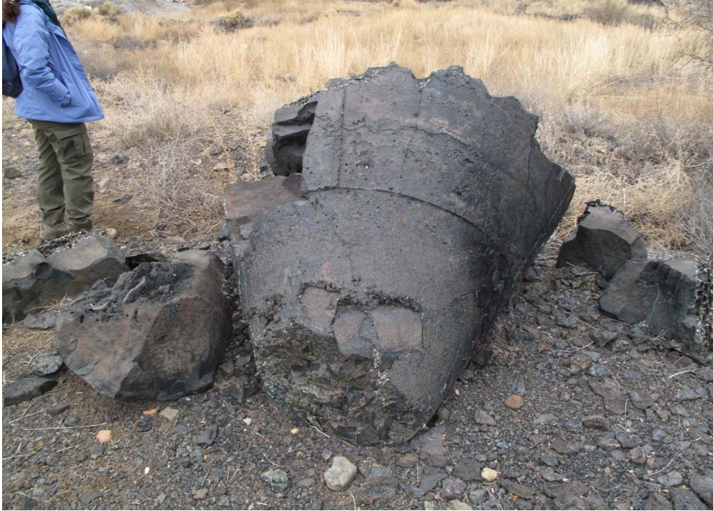
Photograph 33: Slag material dumped in a solid form from the retort or kiln, resulting in a funnel-shaped 3-foot-diameter fragment at VP28
