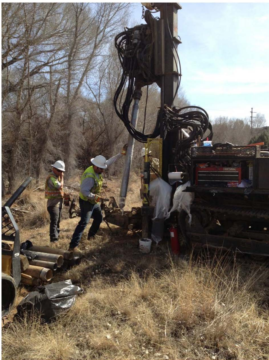
Photo IMG_0814: Photos during investigation: depicting percussive drill rig used to obtain cores from the ground in the Upper Gulch
