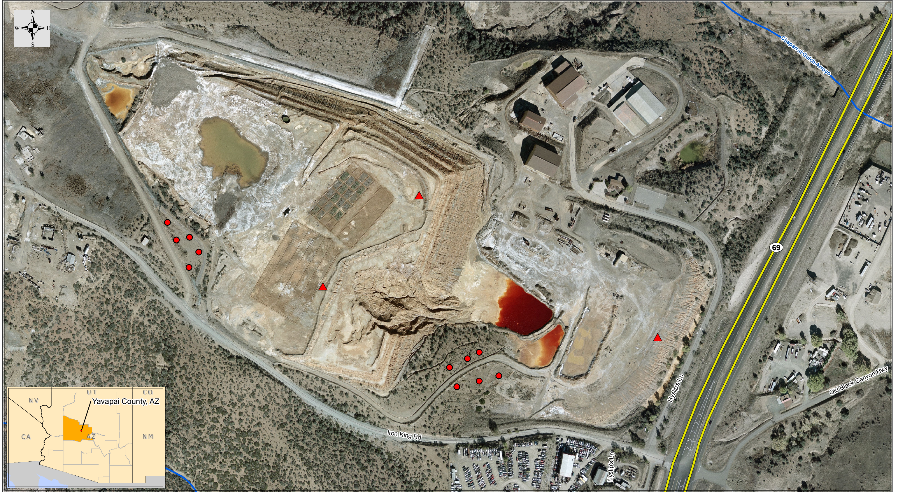
Figure 2 Main Tailings Pile and Adjacent Areas Proposed Borings Iron King Mine Site Dewey-Humboldt, Arizona
